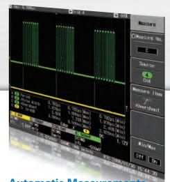
Automatic Measurements Save time making measurements on your signals by using the 26 automatic measurement parameters. See your results color coded to the channels that are being measured. For a more in-depth look turn on the min/max statistics to observe trends in the measurements.
